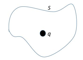
The equation also applies to this surface or any other surface enclosing the charge *q*. Maxwell's 1<sup>st</sup> equation (differential form):
