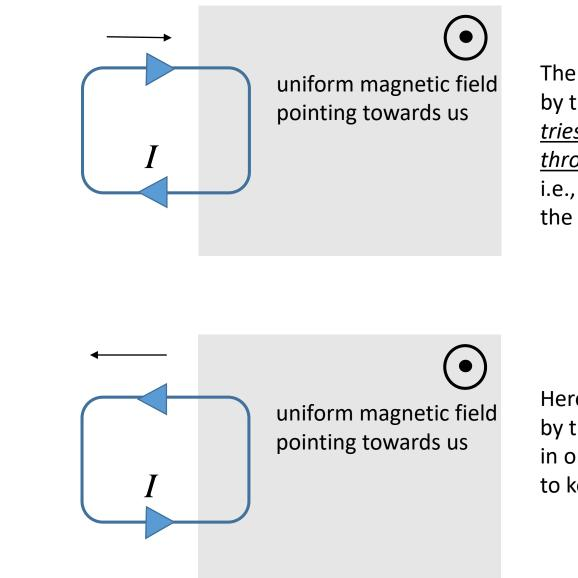
The magnetic field produced by the induced current <u>tries to keep the magnetic flux</u> <u>through the loop constant</u>, i.e., away from us to reduce the increasing flux.
