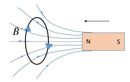
A magnet moving towards a conducting loop induces current in the loop in the direction shown.
