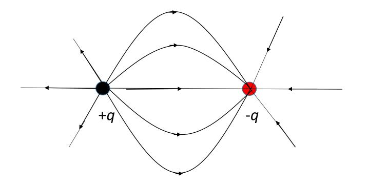
The electric field lines go out of the positive charge into the negative charge.
